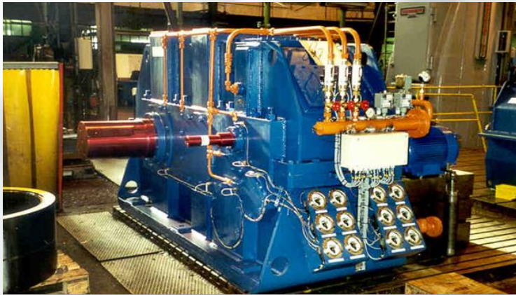
Main gearbox for a cement ball mill
