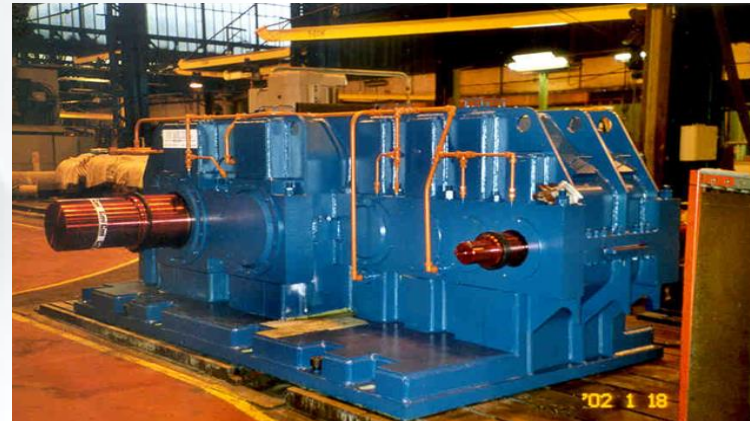
Main gearbox for a cement ball crusher
